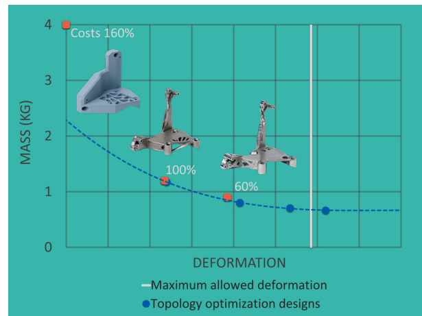
Figure 2 Performance chart of the different designs showing mass versus deformation
