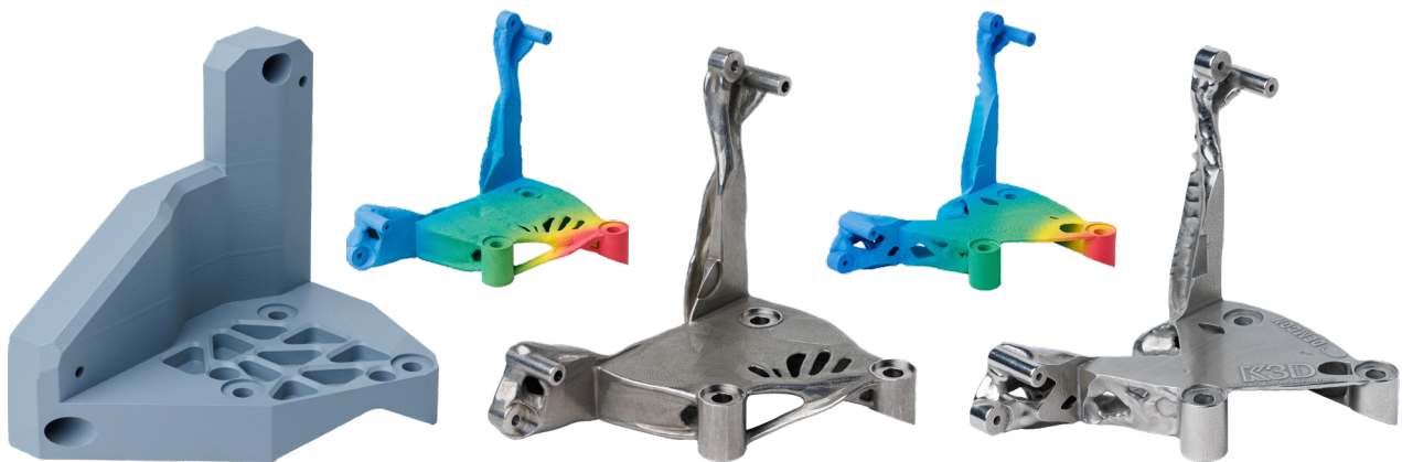
Figure 3 Original design produced by milling and iterations 1 and 2 produced by additive manufacturing
