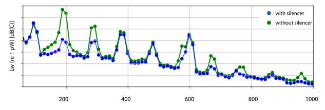
flow through the individual planes was measured, after which the software calculated the total sound power level of the system. For reference the same measurements were performed on an otherwise similar system without the silencer and plotted together for comparison. The chart beneath shows the successful reduction of the peak around 200Hz for which the
