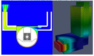
model for cavity resonators was used to find the optimal configuration within the spatial constraints. The final design was verified using an acoustic Finite Element Method (FEM) simulation.
