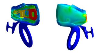
Using computation fluid dynamics (CFD) simulations, we calculated heat transfer in the instrument, while focusing on the casing, the handle, and the motor temperatures.
