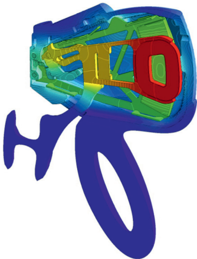
Figure 1 Inside temperature distribution determined with simulations employing a so-called conjugate convective heat transfer model
