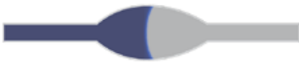
Figure 2 Snapshots of the filling of the microfluidic channel from the left to right. (Blue=liquid, gray=gas & t_0 < t_1 )
